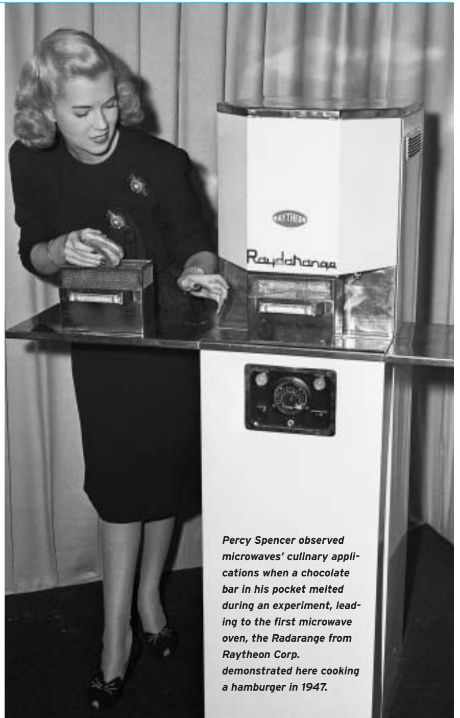
**Percy Spencer observed microwaves' culinary applications when a chocolate bar in his pocket melted during an experiment, leading to the first microwave oven, the Radarange from Raytheon Corp. demonstrated here cooking a hamburger in 1947.**
